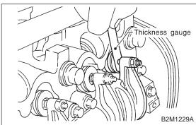
6) Measure #1 cylinder valve clearance by using thickness gauge.
