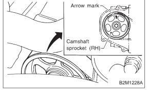
5) Set #1 cylinder piston to top dead center of compression stroke by rotating crankshaft pulley clockwise.
